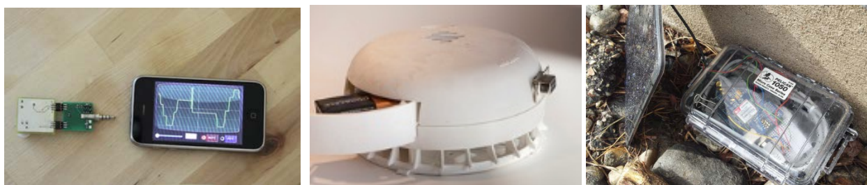
Figure 1. Three types of sensors (left to right): Add-on to cell phones (Project Hijack) 53 , Modified off-the-shelf (UCB-PATS) 54 , and purpose built standalone using existing circuit boards (solar-powered water sensor). 55
